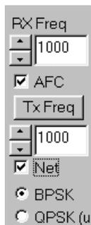
The RX frequency edit control consists of a small edit box where a new frequency can be typed in, or the frequency can be moved up or down using the spin controls just to the left of the edit box. When
