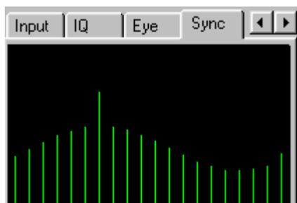
The sync view shows a histogram of the internal signal used to determine the center of the received bit. An elongated line marks the sample that WinPSK is using which is at the peak of the histogram. This display is useful because it can indicate whether the incoming signals bit clock is off frequency (or the users soundcard is off frequency).
