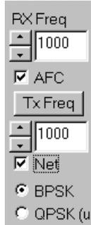
This control activates the Automatic Frequency Control function. It is activated by clicking on the control or pressing the up/down arrow keys. WinPSK will try to adjust the receive frequency to the center of the PSK31 signal.
