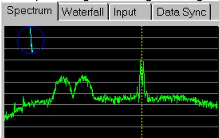
Example of a PSK31 signal that is "Too Wide", probably from being overdriven. There are sidebands only about 15 dB down and the signal is interfering with another PSK31 station just above it in frequency.
